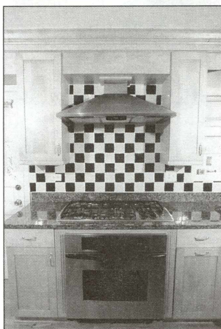
Designer Ross Gerami used a wood chase and stacked moldings to dress up the kitchen and hide plumbing pipes exposed when the soffit was removed.
