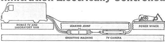
Video Technicians in TV and Laboratory Van control position of TV camera and grouting machine, as well as custom blending of chemical sealants for various leak and soil conditions.
