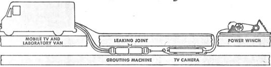
Video Technicians in TV and Laboratory Van control position of TV camera and grouting machine, as well as custom blending of chemical sealants for various leak and soil conditions.
