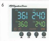
The "COUNTER" on the bottom right shows the number of transfer cycles. It can range from 0 to 999. Press "Reset" for 5 seconds to make counter go to 0.
