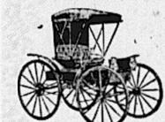
Built for city or country. Will travel ANY ROAD with its 22-inch road clearance. Any speed up to 25 miles per hour. Equipped with a 10-hp. single cylinder motor, 16-12 H.P. No valves, no cams, springs or cam shaft. So simple anyone can RIDE AND KEEP IT RUNNING, never with top, side curtains, storm front, lamps and fall tool equipment.
