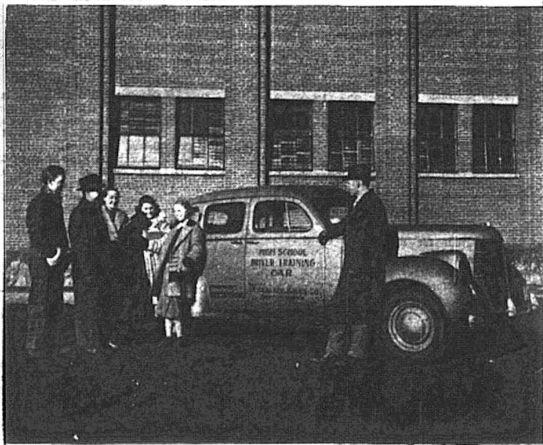
Pictured here is the automobile used by students in Evanston high school's course in "sportsmanlike driving." The car is equipped with two sets of controls, so that the instructor as well as the student, can manipulate brakes and clutch. Similar courses are to be started in many high schools in Illinois and Indiana.
