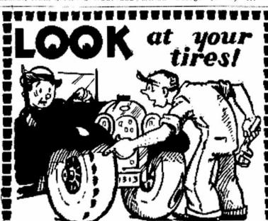
Scuffing, pitting and gouging are due to improper wheel alignment. Ordinary wear—sagging springs, worn bushings, bearings, pivots—throw wheels out of line, drag the tires sideways along the road, scuff and burn the tread, and cut mileage in half.
